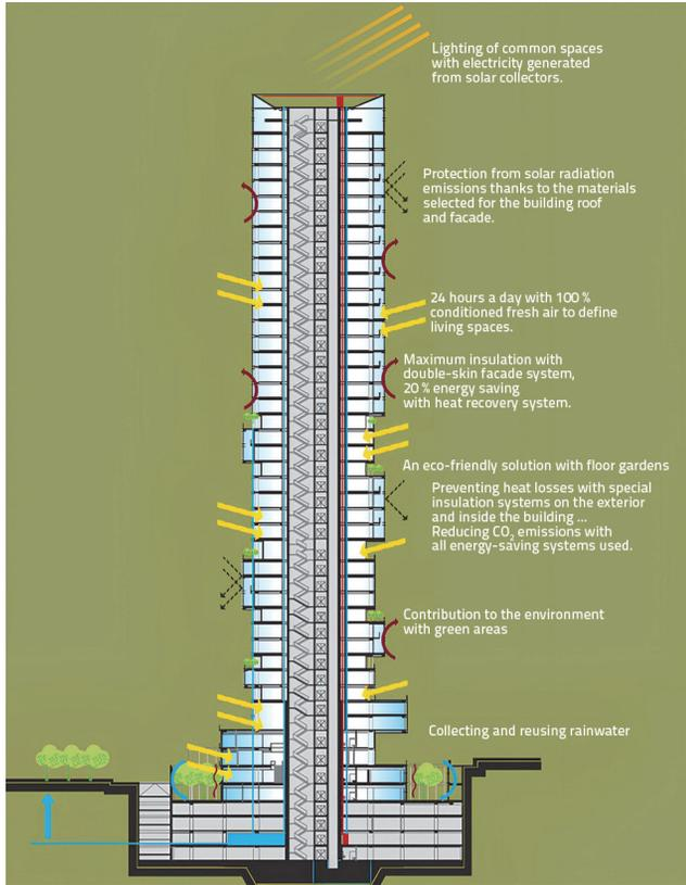
Figure 2. Energy-efficient features of building (modified image [31])
